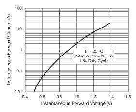
Fig. 3 - Typical Instantaneous Forward Characteristics
