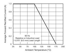
Fig. 1 - Forward Current Derating Curve
