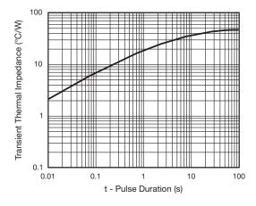
Fig. 6 - Typical Transient Thermal Impedance
