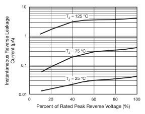
Fig. 4 - Typical Reverse Characteristics
