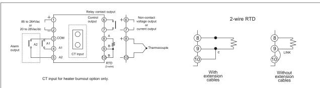
**Notes:** • For ease of connection, especially when using cable trunking, all the terminals are designed to accept wires from the left (when looking from the rear of the unit).
