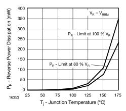
Fig. 5 - Max. Reverse Power Dissipation vs. Junction Temperature
