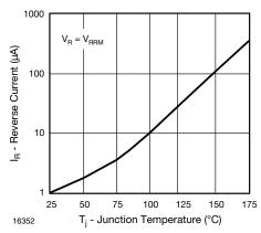
Fig. 4 - Reverse Current vs. Junction Temperature
