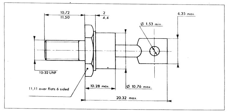
Marking : Cathode connected to case : type number Anode connected to case : type number + suffix R
