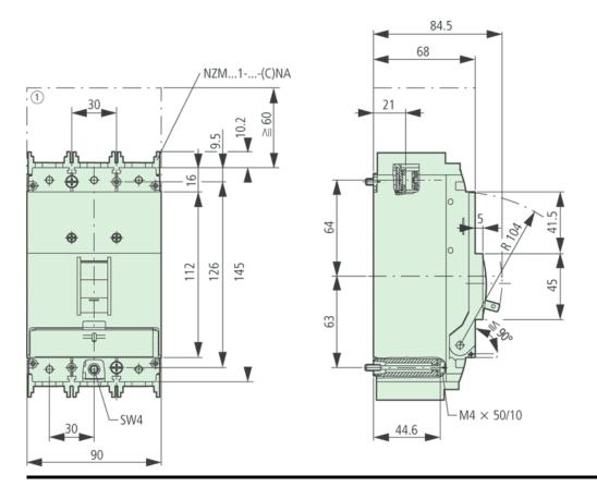
Blow out area, minimum clearance to other parts 60 mm
