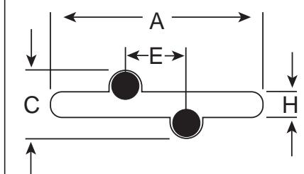
**Table R4. Dimensions for Radial-leaded Devices in Millimeters (Inches)**
