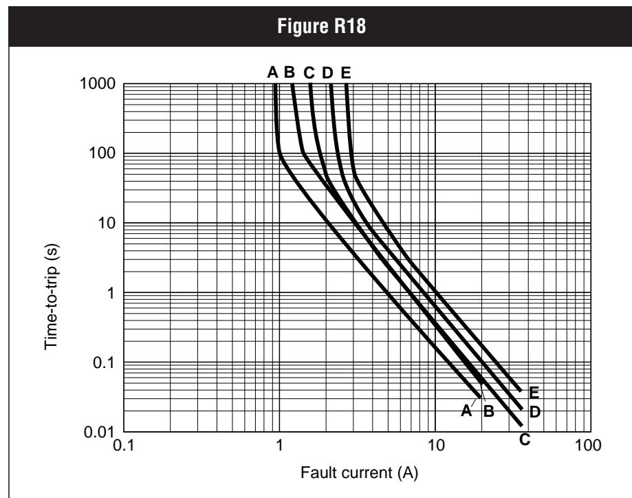
**Figures R17–R23. Typical Time-to-trip Curves at 20°C for Radial-leaded Devices**
