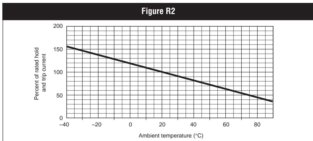
**Figures R1–R5. Thermal Derating Curve for Radial-leaded Devices *continued***
