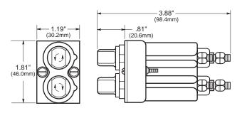
Drilled Mounting Hole Dimensional Tolerance ± 0.005" (0.13 mm)
