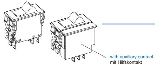
Without release / lock-out latch: code C0
