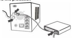
Connect incoming phone line to 'IN' Connect a phone cable from 'OUT' to a modem  $\triangle$  UPS does not provide dial-up function!
