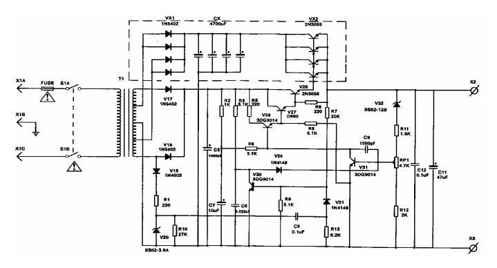
**Note:** The above schematic is for representation of the regulation and output circuit only. The number of filter capacitors, rectifier diodes and 2N3055 output transistors represented in the dotted section, will vary depending upon the output current rating of the specific supply model.
