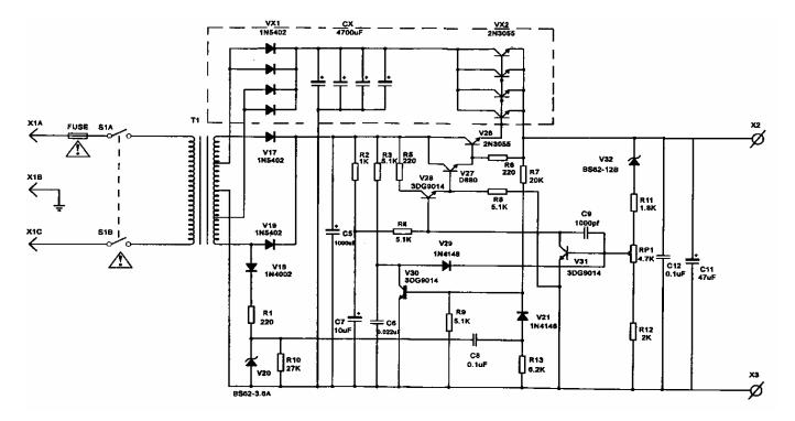
**Note:** The above schematic is for representation of the regulation and output circuit only. The number of filter capacitors, rectifier diodes and 2N3055 output transistors represented in the dotted section, will vary depending upon the output current rating of the specific supply model.
