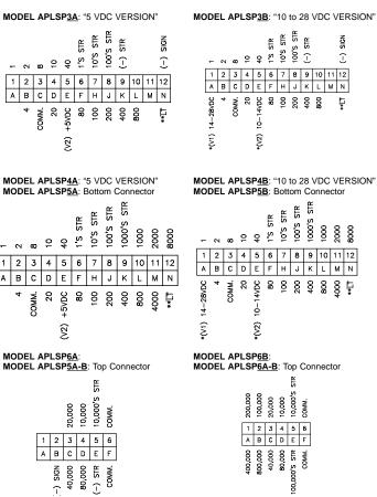
\* Apply power on A and C or E and C.
