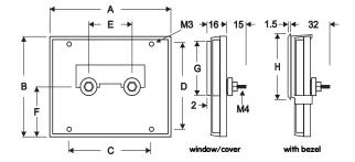
To surface mount, drill 2 x 8mm holes for terminals (and fixing) with centres at dimension E, F and 4 x 3.5mm holes with centres at dimensions C, D (optional).
