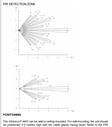
detection patterns shown in Figure 1 when deciding where to position the unit.
