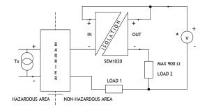
Used to increase the limited drive capability of a intriniscally safe (4 to 20) mA loop
