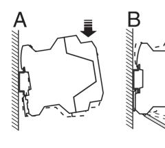
The assignment of the connection terminal blocks is shown in the block diagram. The module can be snapped onto all 35 mm DIN rails according to EN 60715.
