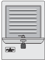
Protection for ventilation openings (i.e. pressure compensation)
