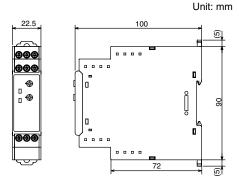
\*Installation Procedure: Mount to the DIN Rail or with front screws \*Dimensions for Mounting with Front Screws
