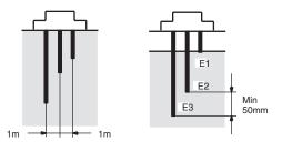
Electrodes are in actual contact with the liquid. Standard electrodes are made of stainless steel and usable in purified water, sea water, sewage, acid (except acetic acid, sulfuric acid, etc.) and alkaline liguids, although they may corrode depending upon the temperature and working conditions.
