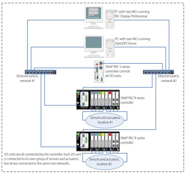
This diagram shows a SNAP PAC S-series controller connected to two separate Ethernet networks. This configuration addresses the concern that an Ethernet network may fail or need maintenance, leaving the PC running OptoOPCServer, the PC running PAC Display, the controller, and the I/O units unable to communicate.
