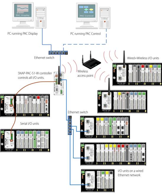
The Wired+Wireless SNAP PAC S-series controller is controlling three groups of I/O units: one group through its serial port, another through a standard 10/100 Mbps interface, and the third over a wireless LAN.
