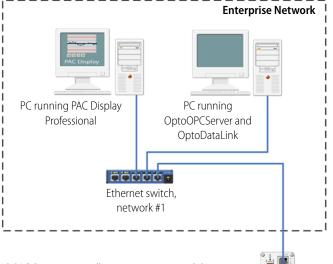
This diagram shows multiple Opto 22 SNAP I/O units connected together over an Ethernet network and controlled by a SNAP PAC S-series controller running a control strategy. The controller is also connected to a larger, separate enterprise Ethernet network to provide data to two PCs running Opto 22's PAC Display HMI software and OptoOPCServer.
