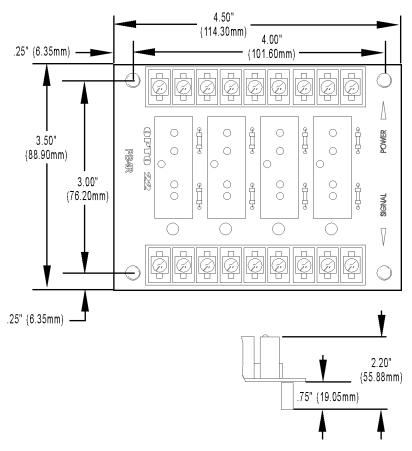
**Note:** The PB4R has only 4-pin connections, NOT 5-pin.
