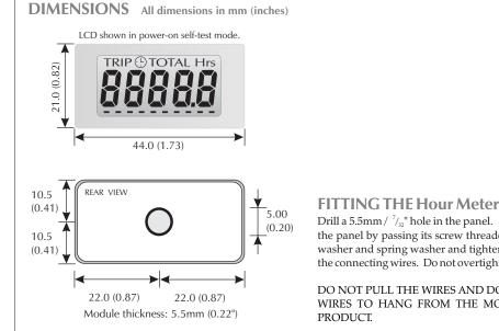
Drill a 5.5mm/ $^{7}/_{32}$  hole in the panel. Fit seal to the rear of the module. Fit the module to the panel by passing its screw threaded stud and the wires through the hole, fitting the washer and spring washer and tightening the nut provided. Take care not to trap any of the connecting wires. Do not overtighten the nut as this may damage the meter.
