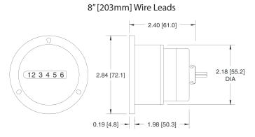
Mounting holes: For #4 screws on 2.44" [62.0] B.C. and #6 screws on 2.53" [64.3] B.C. Panel cutout: 2.21" [56.1] Dia.
