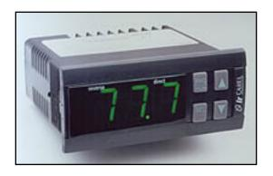
The IR32 series of general purpose Controllers, with their Analogue, Thermocouple and RTD input and Relay or SSR drive output options, combine simple control and programmability with flexibility of use for a wide range of applications. They are available with 1, 2 or 4 outputs/Set-points, can be configured for 9 different control modes for On/Off, P or PI action and used to control Temperature, Humidity, Air-pressure or other media with suitable transducers.
