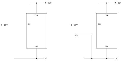
Measuring a voltage source with a common signal and supply ground
