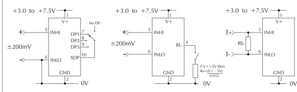
Measuring a single ended input voltage referenced to supply, i.e. the input voltage and the meter's power supply share the same 0V rail. Ensure solder link LCOM is open.
