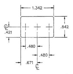
NOTE: A template can be made to these dimensions; or the 3 screw holes can be drilled (as per the instruction sheet) on these centers.
