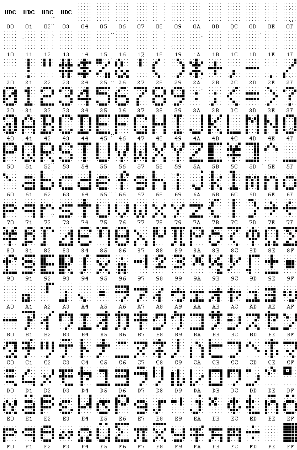
Figure 3-9 Hitachi (LCD) Character Set
