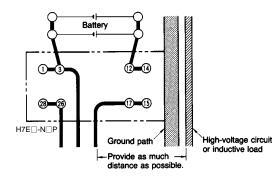
Be careful not to apply voltages exceeding the following values to the count, timer, or reset terminals, otherwise the internal circuit may be damaged.
