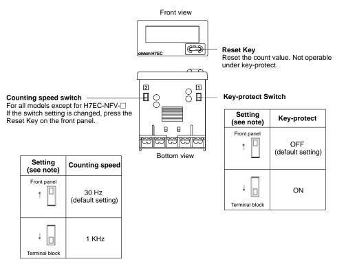
Note: Perform switch setting before mounting to a control panel.
