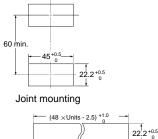
Waterproofing is not possible for joint mounting
