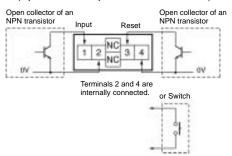
Note: 1. Residual voltage in the output section of Proximity Sensors or Photoelectric Sensors becomes less than 0.5 V because the current flowing from terminals 1 or 3 is as small as approx. 10 μA, thus allowing easy connection.
