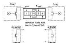
Note: Use Relays and Switches that have high contact reliability because the current flowing from terminals 1 or 3 is as small as approx. 10  $\mu$ A. It is recommended that OMRON's G3TA-IA/ID be used as the SSR.
