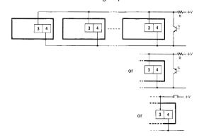
Note: H (Reset ON) level must be 4.5 V minimum.
