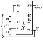
Using the formulae choose resistors to ensure the analogue inputs are no closer than 1.5V from either VDD or VSS (VDD-1.5V or VSS+1.5V)
