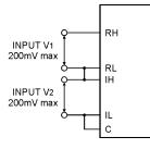
To determine the ratio between two voltages apply the inputs as shown. Displayed reading =  $\frac{V2}{V1} \times 1000$
