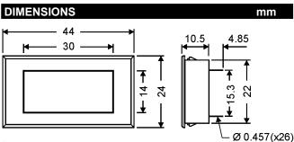
Panel cut out 40.5 x 22.5 Fastening clips accept panel thickness 0.9 to 3.2mm
