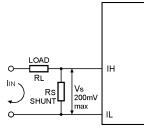
Shunt resistance Rs =  $\frac{Vs}{IIN} \Omega$
