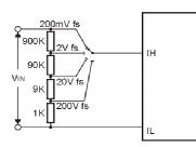
For multi-range, use a 2 pole, 4 way rotary switch. 1 pole for range select and the other to connect the appropriate decimal point to XBP.
