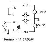
To achieve a zero display reading for a non-zero voltage input, apply the offset voltage between C and IL. For a positive offset apply a Positive signal to IL w.r.t. C. Apply the input signal between IH and C Note jumper J1 must be open
