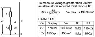
The input impedance becomes R1+R2. Choose accurate stable resistors. Typically, R1=1M $\Omega$ . 9M $\Omega$  is a practical upper limit.
