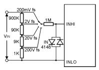
For multi-range, use a 2 pole, 4 way rotary switch. 1 pole for range select and the other to connect the appropriate decimal point to XBP.
