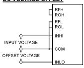
To achieve a zero display reading for a non-zero voltage input, apply the offset voltage between COM and INLO.
