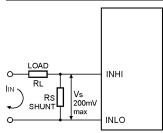
Shunt resistance Rs =  $\frac{Vs}{IIN} \Omega$
