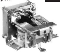
The circuit selection wiper on Electrical Reset Steppers can be reset to zero or the home position from any desired position by energization of the reset magnet. One of the most versatile and widely used steppers in the Guardian line, the ME offers smooth and reliable performance - proven in thousands of applications. The interlock arraingment between the reset and step magnets allows the MER to perform some of the functions of an interlock relay.
