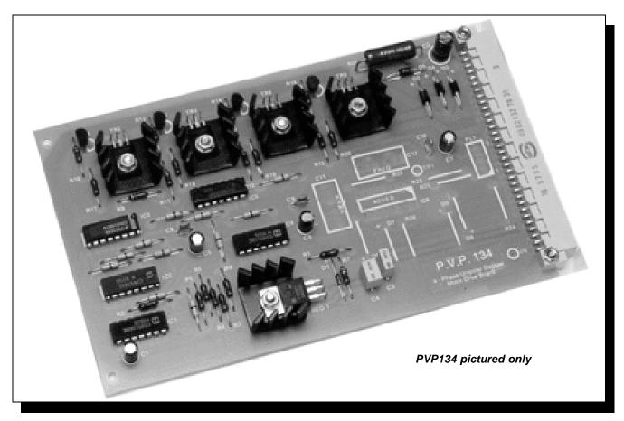
The Series 13 range of Stepper Motor Drives, manufactured by Alzanti, have been developed to meet the growing demand for high performance, cost effective, L/R drivers. They have been designed to be compatible with the specifications of many permanent magnet and hybrid stepper motors up to NEMA frame size 34 and are therefore suitable for numerous applications.
