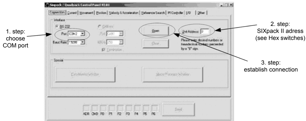
Figure 5.5: Setup of SQPack
