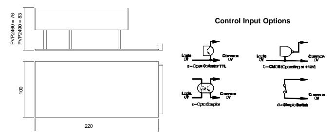
NOTE: PVP2490 has a force cooled heatsink assembly fitted
