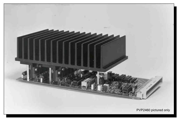
The Series 24 range of stepper motor drives, manufactured by Alzanti, have been developed to meet the growing demand for high performance, cost effective, bipolar drivers. They have been designed to be compatible with the specifications of many stepper motors, with options available to suit numerous applications. PWM chopper regulation provides a very efficient motor drive stage, extending the useful speed range of motors whilst reducing heat dissipation and power consumption.
