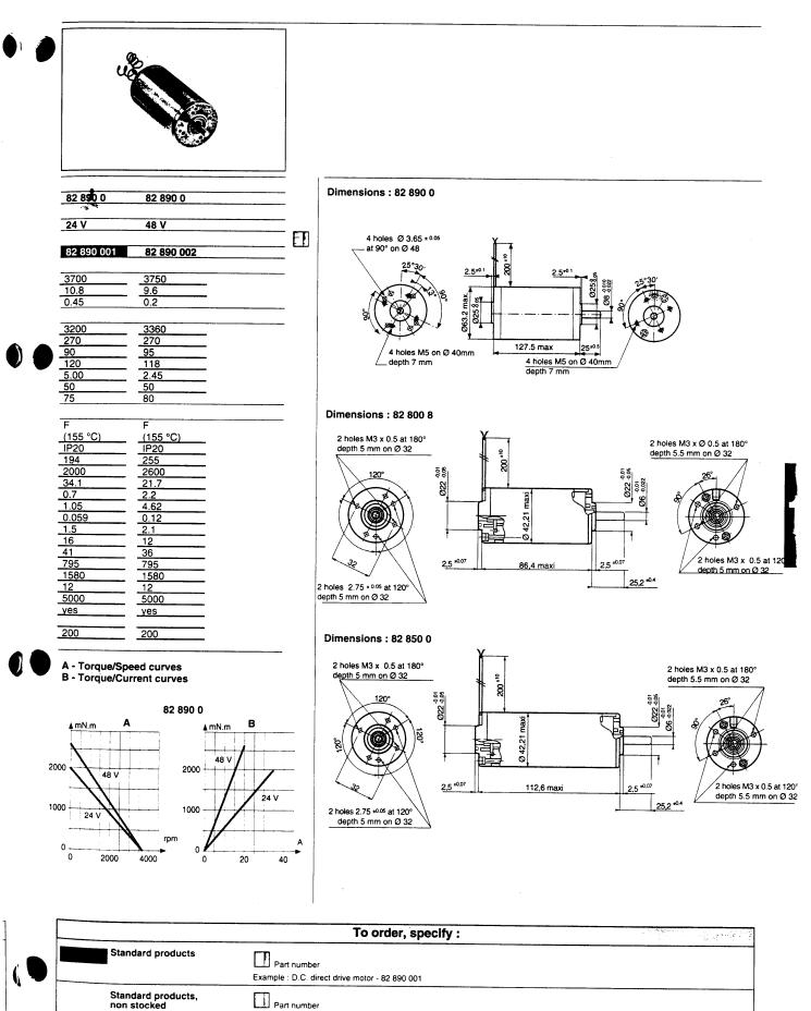
Example : D.C. direct drive motor - 82 800 802 - 24 volts
