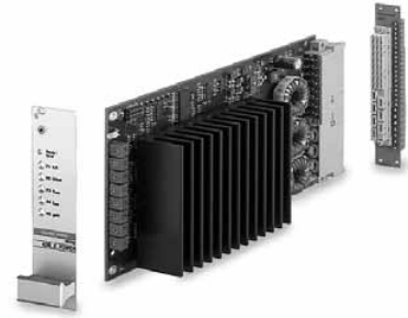
ADS_E 50/10 4-Q-DC Servoamplifier Powerful PWM servoamplifier for permanent magnet activated DC motors from 80 to approx. 500 watts output power. Available as Power Version in Eurocard format.
