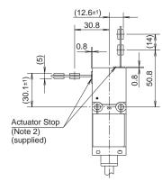
• Using the HS9Z-A62 Right-angle Actuator
