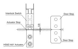
When using horizontal/vertical angle adjustable actuator (HS9Z-A65/A66)
