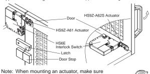
that the actuator enters the slot in the correct direction, as shown on the right.
