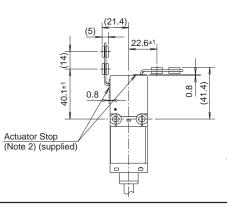
Using the HS9Z-A65/A66 Angle Adjustable Actuator (25) 22.6±1 28.8 0.8 (25) 48.8 0.8 Ŧ <u>ى</u> Actuator Stop (Note 2) (supplied) Ŵ
