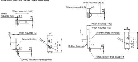
Note: The actuator stop is used to adjust the actuator position. Remove the actuator stop after the actuator position is mounted.
