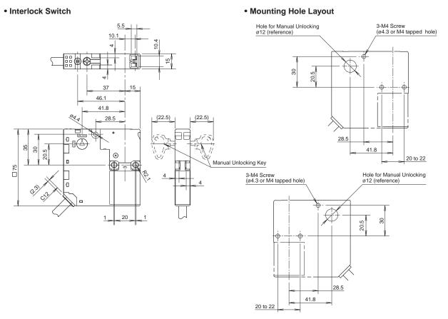
When using straight actuator (HS9Z-A61) When using right-angle actuator (HS9Z-A62S)
