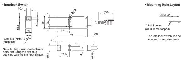
• Using the HS9Z-A61 Straight Actuator
