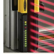
LEDs and 7-segment display indicate system status, alignment and blocked beams.
