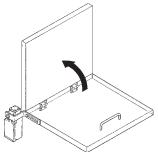
**Note:** Install the arm lever so that it will not rotate more than 180°.
