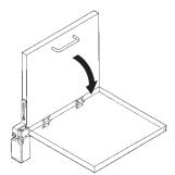
**Note:** Install the arm lever so that it will not rotate more than 90°.
