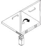
**Note:** Install the arm lever so that it will not rotate more than 180°.
