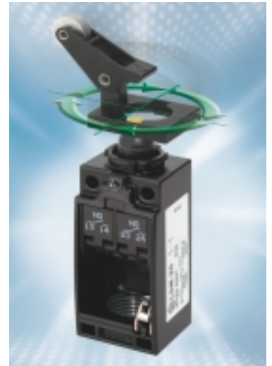
The operating head can be attached in all four directions (4 x 90°) and can be installed quickly and securely with a bayonet fitting.
