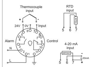
**Note :** When pin 11 and the sensor are both earthed, the DTC410 will display OPN and will not operate correctly. For 24V models use an isolated or non-earthed sensor.
