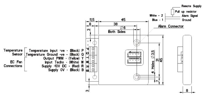
Note: for ebm-papst EC fans without an integrated 10 volt supply, please refer to the EC Fan Controller User Guide (980-OMI10740) for alternative wiring of the supply.
