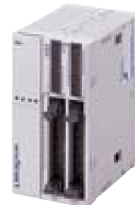
FC4A-D40K3 24 input points 16 output points 0.3A transistor sink output 24V DC 31.2KB memory 264 max I/O expandability
