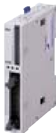
16-point Transistor Source Output Module FC4A-T16S3 16 output points 0.1A transistor source output MIL connector
