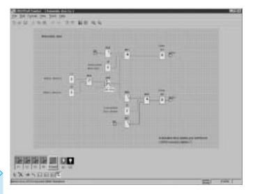
Easy program design is only part of the solution. To make startup even easier, LOGO!Soft Comfort offers a powerful simulator that lets you quickly examine the program operation. You can activate inputs, monitor timers and counters, even simulate a power cycle! Once your program is operating the way you want, simply connect the PC cable and download the program.
