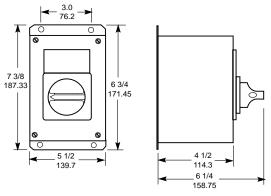
NEMA Type 4, 4X, 12 (V1W30, V2W30, V1A30, V2A30)
