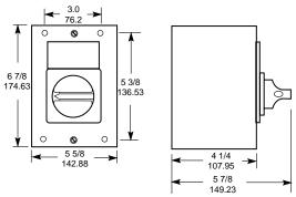
Metallic Enclosed Switch: NEMA Type 1 (V1G30, V2G30)
