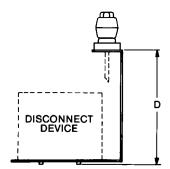
Note: Back panel support is recommended for Types TFB1, 2, and 3. Other devices may also require support if flange is not sufficiently rigid.
