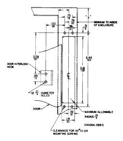
**Panel Drilling for Alternate Mounting Method**
