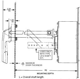
H = Distance from inside of enclosure door to circuit breaker mounting surface.
