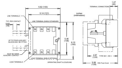
Drilling Dimensions for 9421 NW2/NW2B
