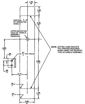
Enclosure Door Cutout and Door Interlock Hook Mounting Dimensions
