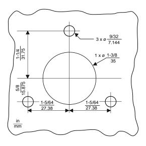
Panel Drilling for 9421 LC and LH Handles
