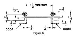
(1) ¼ Drill in Leg of Inside Door Channel at ¢ of Vault Handle.
