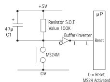
Inverter input held at 0V (logic 0) with no disturbance, a charge is permanently held in CI. With movement the MS24M goes momentarily open circuit allowing the charged capacitor to be seen at the inverter input which would change state giving a pulse to reset.
