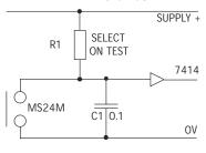
The output of the MS24M may be damped when less sensitivity is required by using a Schmitt trigger device as shown. Lowering the value of R1 (100 ohm min) will reduce the sensitivity of the switch.
