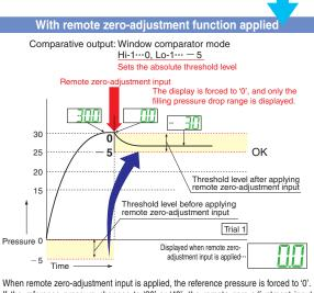
If the reference pressure changes to '20' or '40', the remote zero-adjustment input adjusts the reference pressure to '0' every time the reference pressure changes, so any variation in the filling pressure can be ignored.
