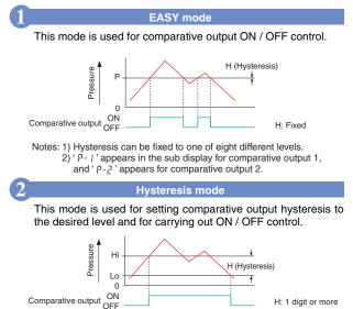
Note: '  $H_{I} = I$  ' or '  $L_{D} = I$  ' appears in the sub display for comparative output 1, and ' $H_{I} = 2$ ' or ' $L_{D} = 2$ ' appears for comparative output 2.
