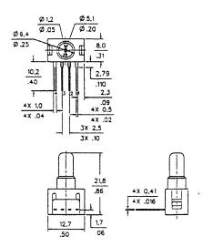
DIFFERENTIAL SENSOR Straight Port, 1 x 4 termination (Style 2) ONLY Port P1 is near terminals.
