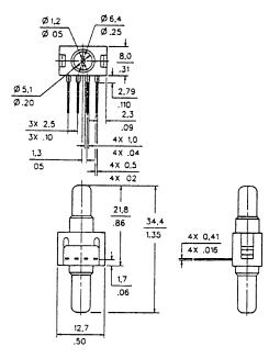
"2 x 2" Termination (Style 2), Port Style A, Straight Pin 1 is notched, and is shown at lower right corner. Pins 2, 3 and 4 are clockwise.
